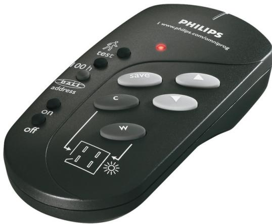
IRT8097/00 Simplified commissioning tool for OccuSwitch DALI, for light level calibration, window/corridor programming and installation test.
