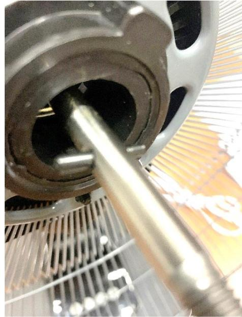
*Pins on the motor shaft*
